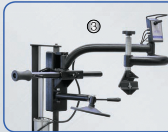
(1) Powerful bead breaker (2) Fine adjustment by joystick (on the mounting arm) (3) Help-arm with bead roller, bead presser and bead loosening disk (4) Large air tank for the integrated air boosters in the mounting jaws
